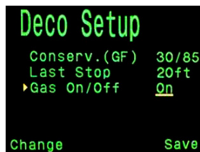
Enabling Gas On/Off mode
